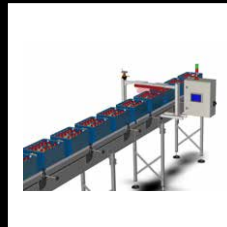
QUANTUM Arca Crate fill-level monitoring
